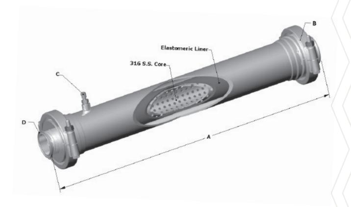
The Silencer™is installed directly into your product line as close as possible to the source of the pulsation (i.e. typically at the discharge of a homogenizer or prior to a filler). Once installed the unit is charged with a gas (typically plant air) to 10-15 psig. Reverse osmosis systems should be charged at 90-100 psig. The Silencer™ is completely cleaned in place (CIP) by normal procedures.
